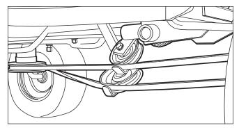
Figure 9. Front Idler Pulley Installed
